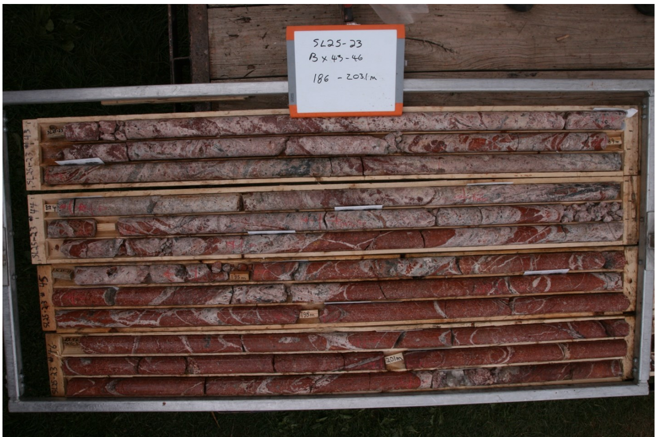
Figure 2. High-grade carbonatite mineralization with grades up to 8.67% TREO over 1.5m in borehole SL25-23.
