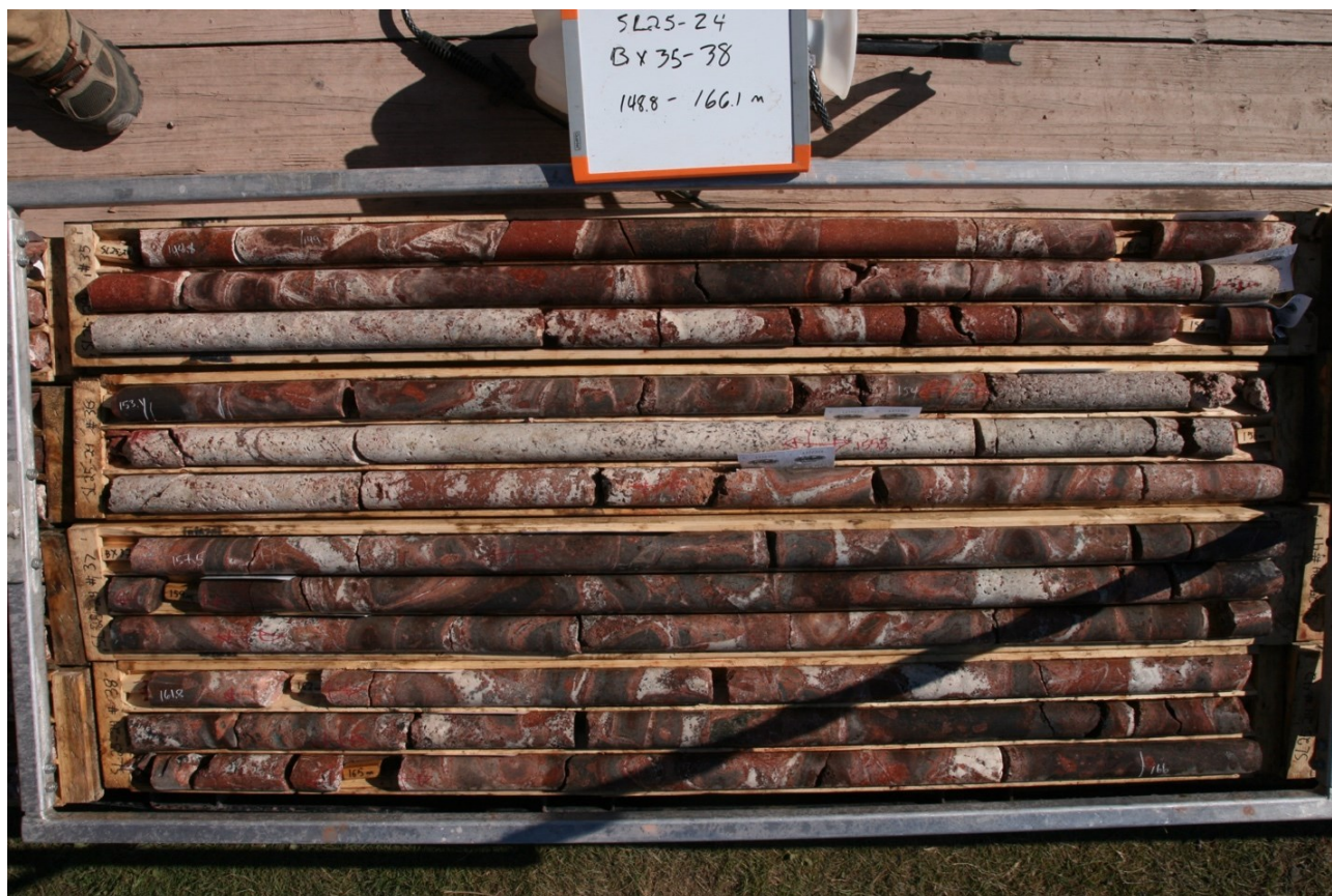
Figure 2. High-grade carbonatite mineralization with grades up to 5.21% TREO over 2.5m in borehole SL25-24 (155.5 – 158.0m).
