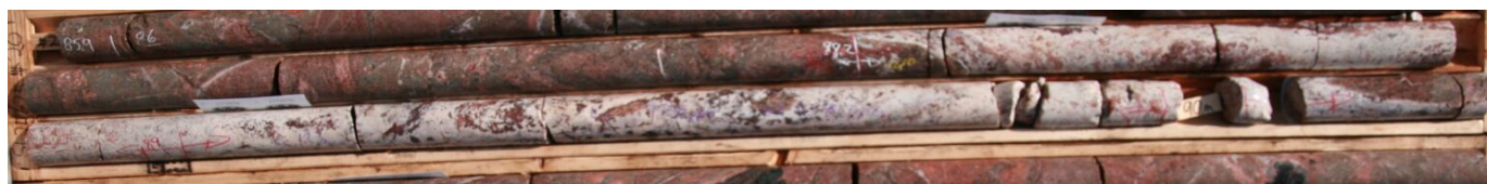
Figure 3: Core photo of drill hole SL25-25, 88.2–90.4 m (2.20 m), showing white vuggy carbonatite vein with red hematite and purple fluorite in hematitized red syenite.
