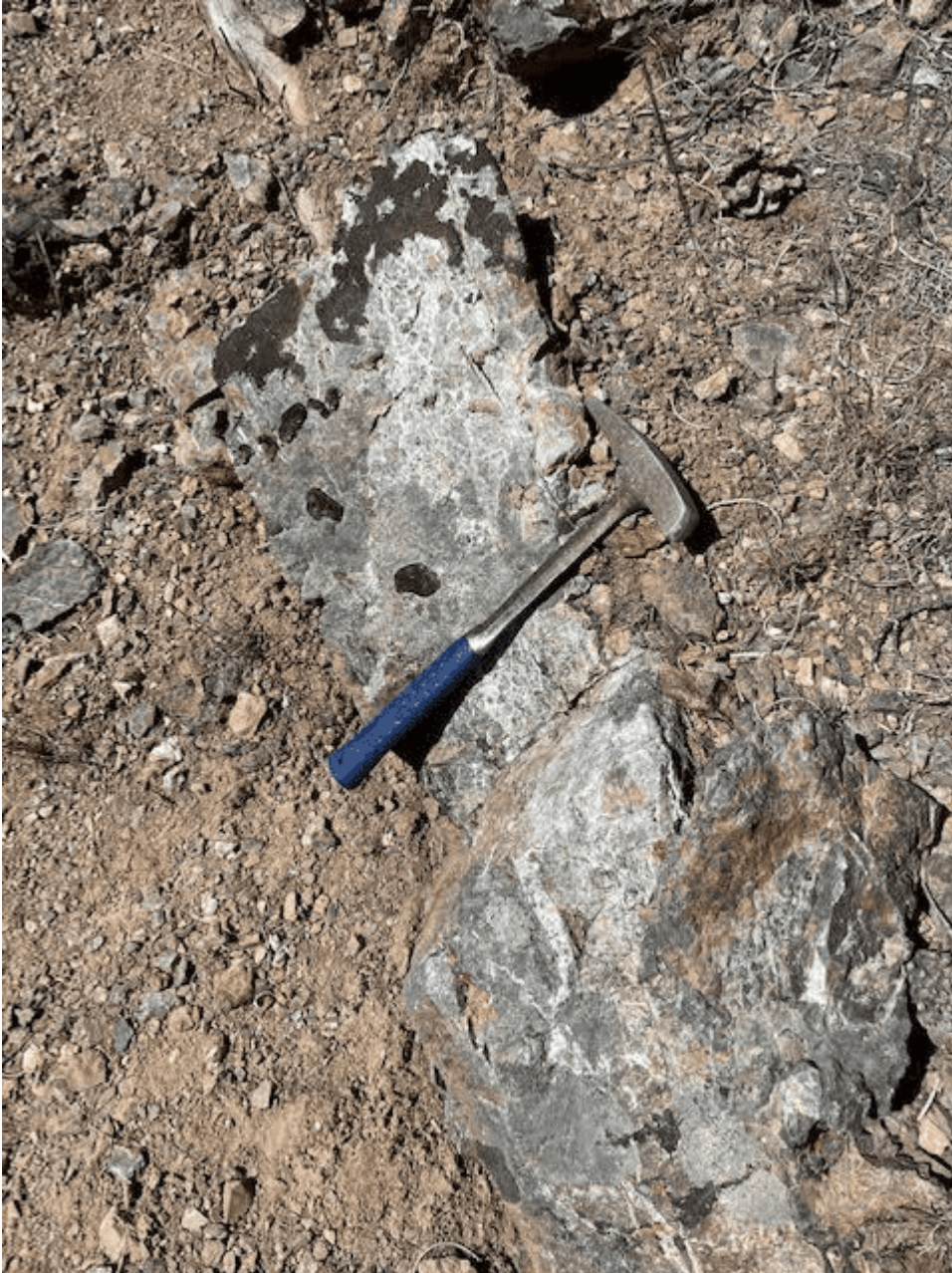
Figure 4: Target Drill Site Cut Exposing a Clay-Altered and Oxidized Igneous Dike within the TH Fault
