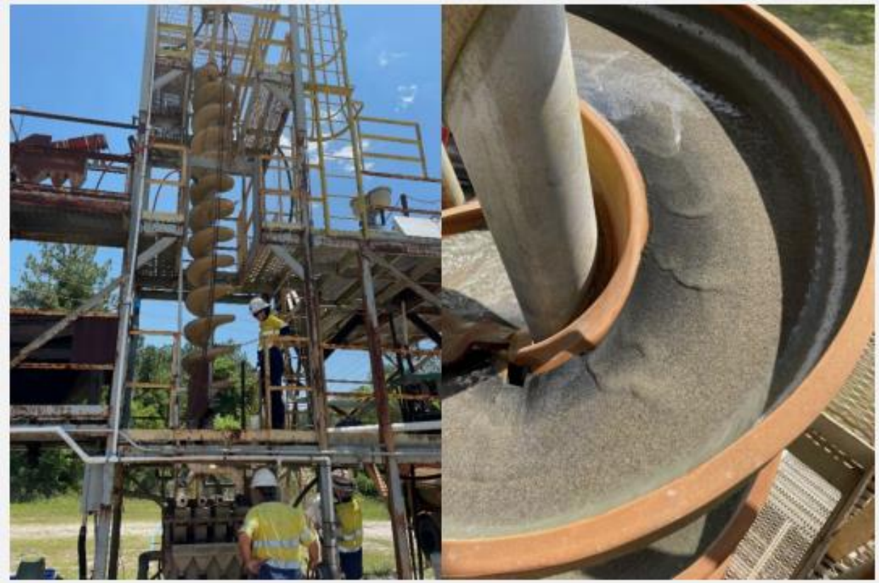
Figure 4 – MG 12 Spiral from Mineral Technologies and Halleck Creek Feed in the Spiral
