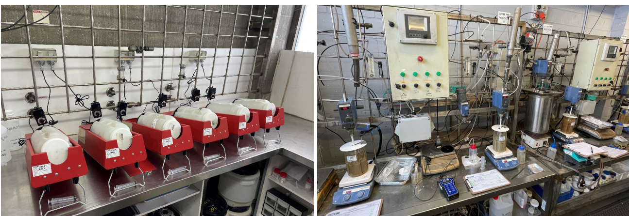
Above: Core Resources have been conducting testwork using multiple atmospheric leaching methods, including bottle roll tests (left) and tank leaching (right). Testwork will continue in Q1 2025.
