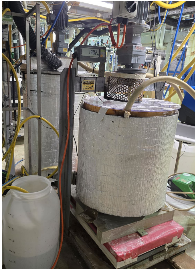
Above: A 200kg bulk leach was carried out on a composite of 137 drill core intervals at ANSTO.
